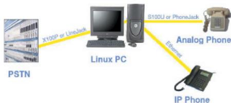
process both data and voice – and the nature of Asterisk’s modular design allows for extensive customization. For instance, dial plans for extensions can be configured to route traffic to either digital or analogue endpoints, including phones.
